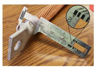
\* Avoid the embossed lettering when measuring the crimp as this area could yield an incorrect reading.
