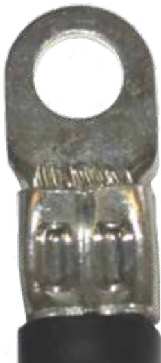
Close up of "M" Profile Crimp
