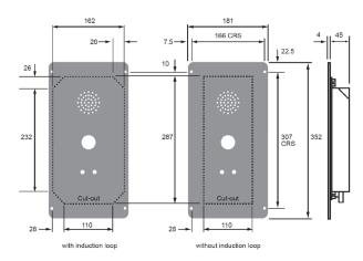
Note: Rear enclosure dimensions approx. W186mm x H366mm x D60mm
