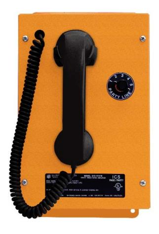
ICS operation is simple; the user lifts the station handset, presses the page pressbar and announces. The responding individual lifts the handset of their nearest station for full duplex communication over the party line.
