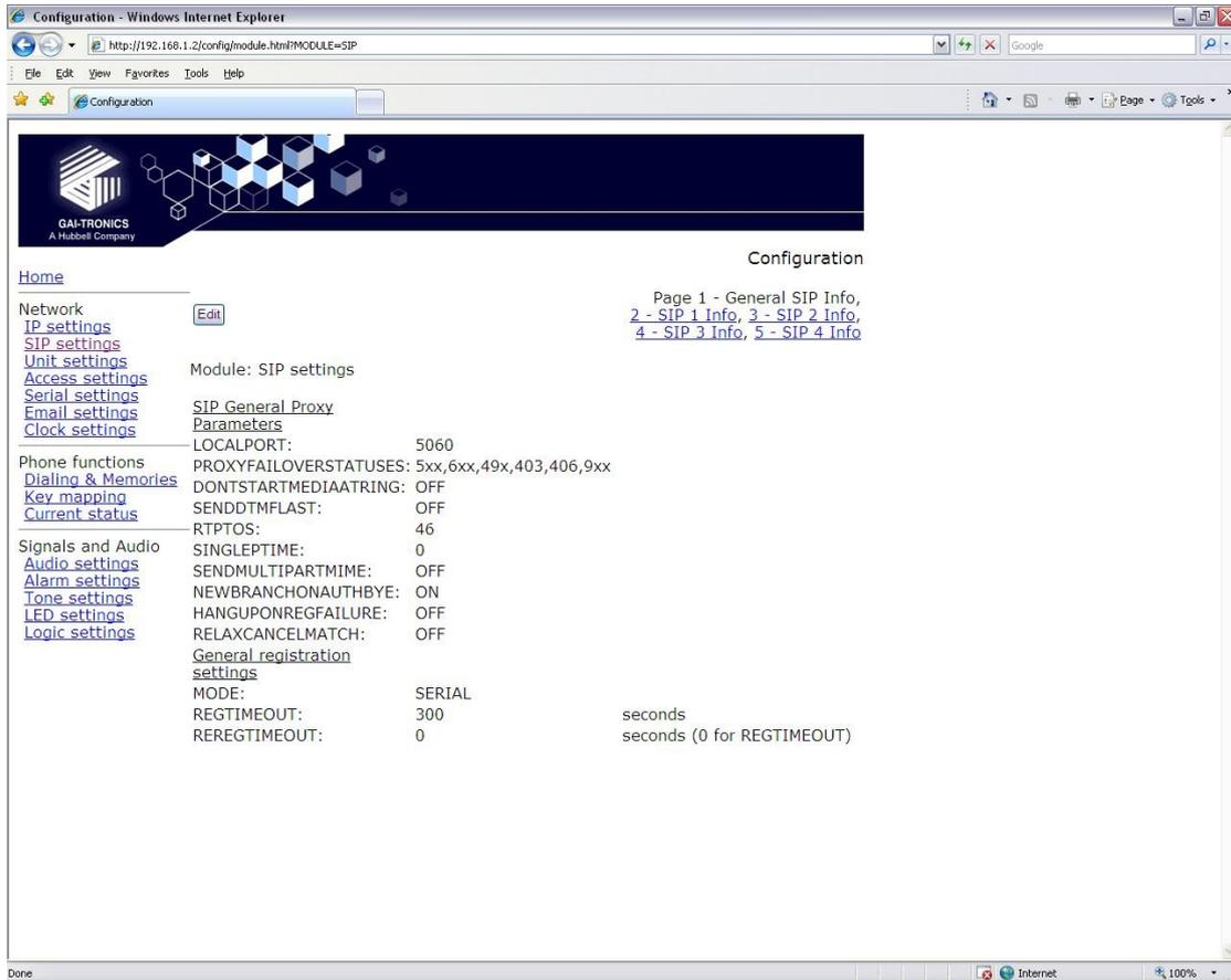
**LOCALPORT:** Configures the port number used for the local SIP signalling socket.
