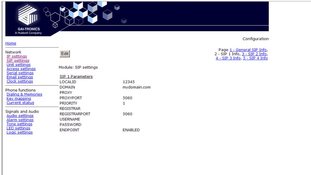
Each of the 4 sub pages is identical, and is used to set parameters for each of 4 possible proxies.
