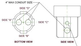
MAX DIA OF SECOND CONDUIT TAP IN SIDE WALL IS 2 1/2"
