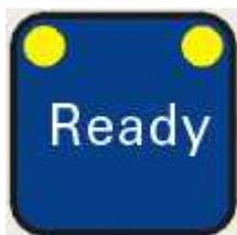
First you have to press the *Ready* button to bring the system into ready state. If this action succeeds and the system switches into ready state it indicates this by changing the colour of the digits in the output voltage and current display from grey to black. If the system can not switch to ready state please check the alarms.
