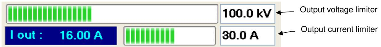
The limit value of the *output voltage* can be set between 0 kV and the maximum possible voltage of the taps or the circuit variant.
