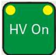
When the system is in ready state High Voltage can be switched on by pressing the *HV On* button. This closes the secondary breaker (K2) of the regulating transformer. The secondary breaker of the regulating transformer is the HV relays.
