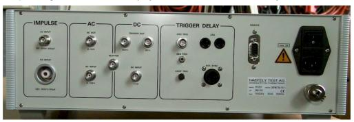
Fig. 43a: Rear side of DMI551 with measuring channels
