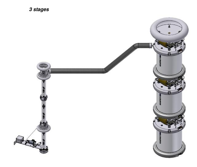
Fig. 65: Build-up AC configuration 3 stages
