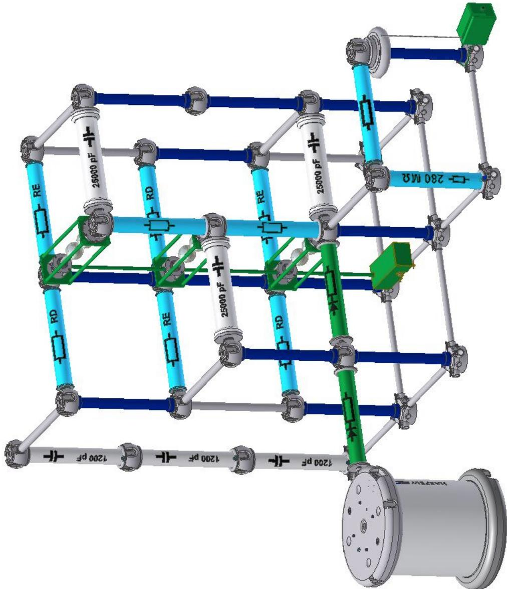
Fig. 71: Build-up Impulse configuration 3 stages
