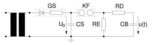
Fig. 51: Circuit for generating impulse voltages
