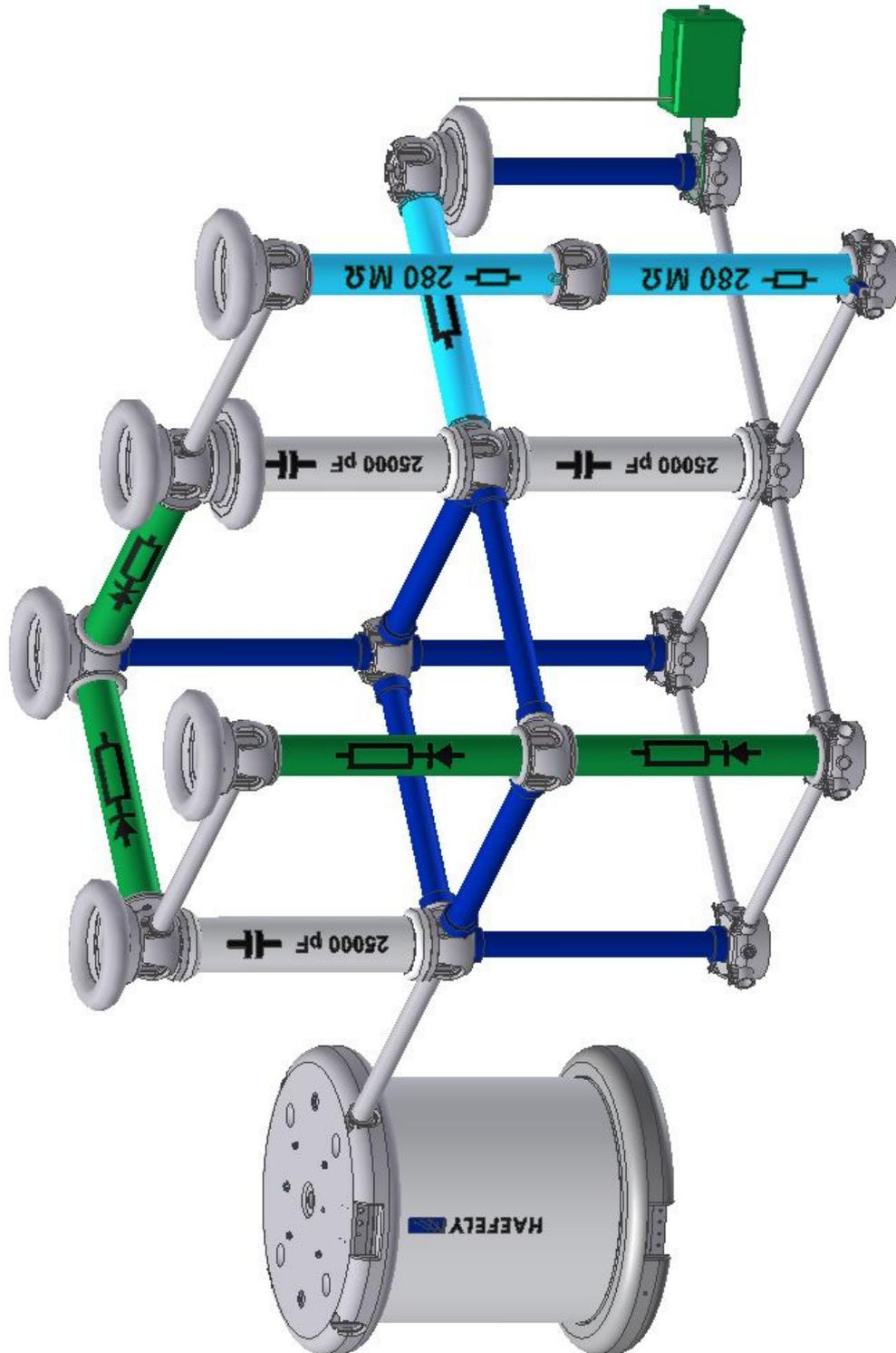
Fig. 67: Build-up DC configuration 2 stages
