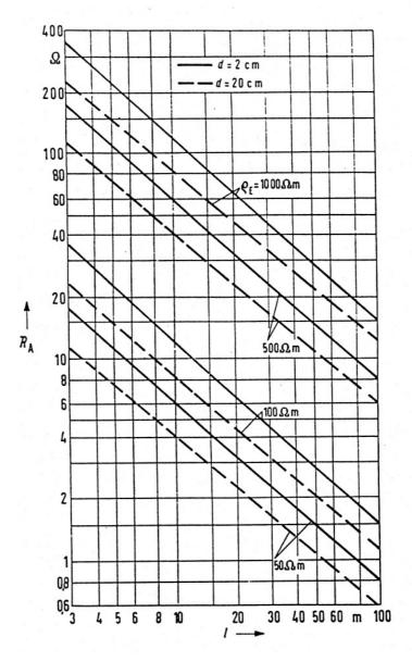
Figure 54 shows the grounding resistance as a function of length of rod and soil resistivity
