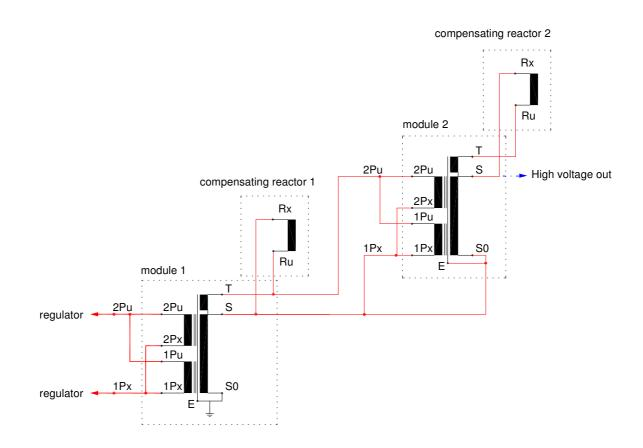
Fig. 58b: Schematic 2 stages with compensating reactors
