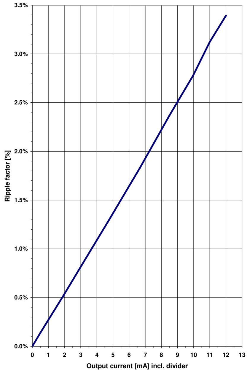
Diagram 4: Ripple factor DC 2 stages
