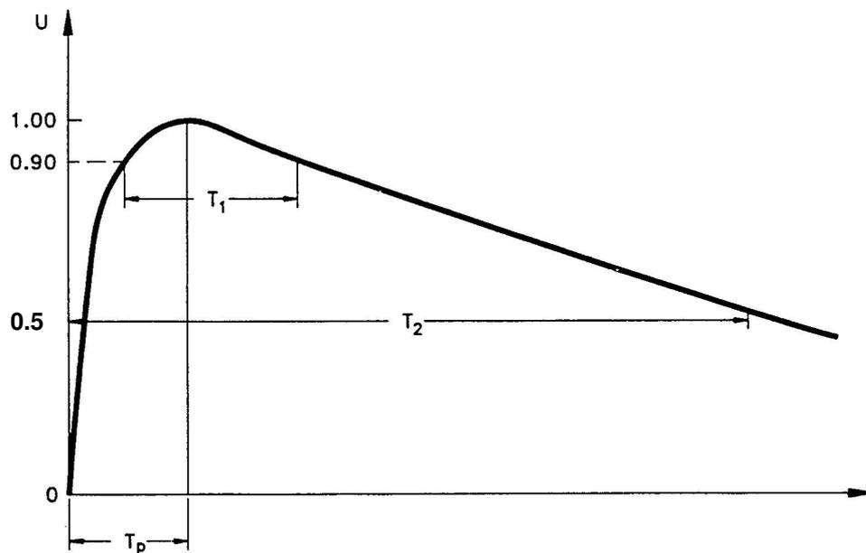
Fig. 50. Switching impulse curve
