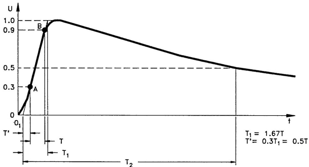
Fig. 49. Lightning impulse curve
