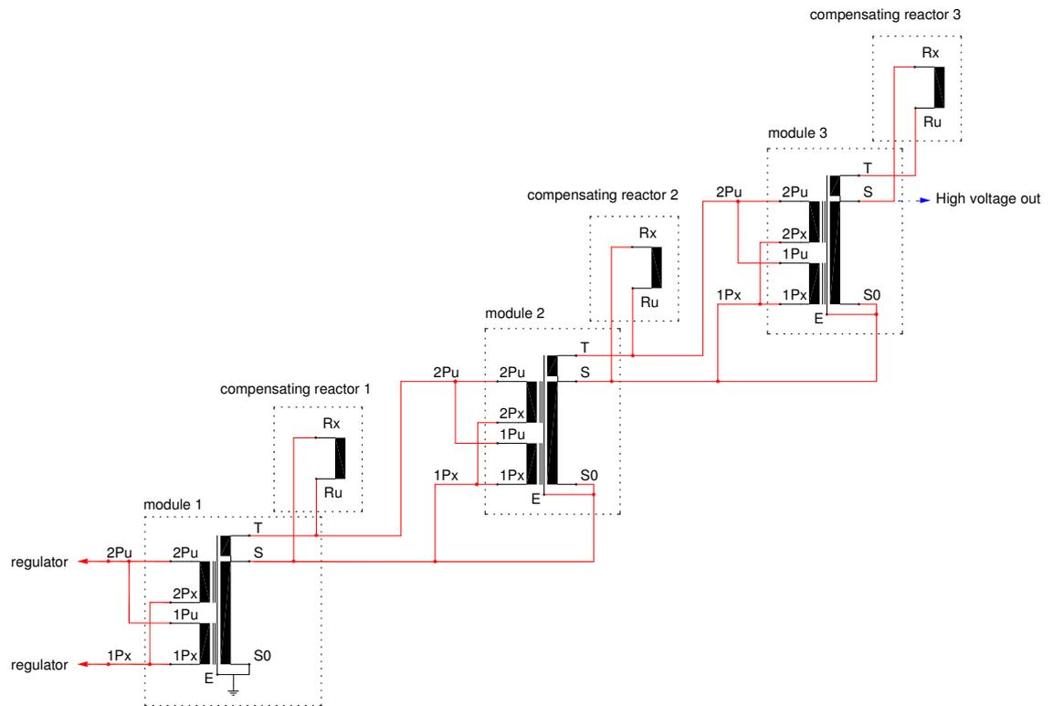
Fig. 62a: Schematic 3 stages with compensation reactor
