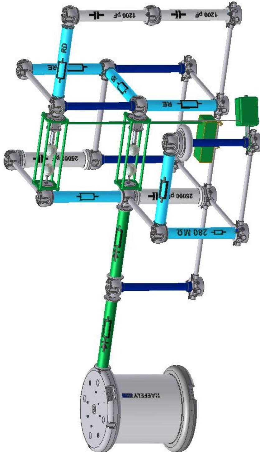
Fig. 70: Build-up Impulse configuration 2 stages
