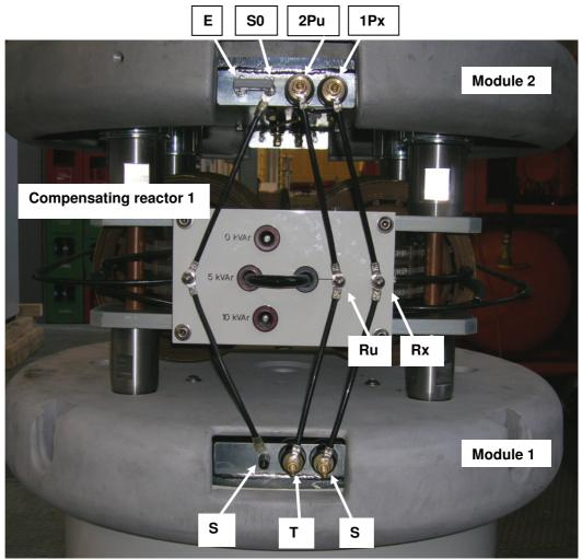
Fig. 61b: Connections between the two modules and the compensating reactor
