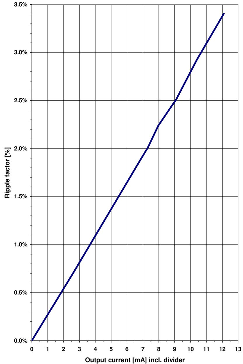
Diagram 2: Ripple factor DC 1 stage
