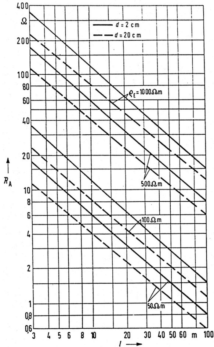
Fig. 54: Grounding resistance as a function of length of rod and soil resistivity
