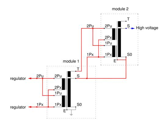
Fig. 58a: Schematic diagram for cascade connection of two test transformer
