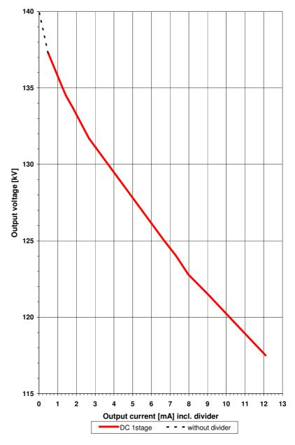
Diagram 1: Load range DC 1 stage With divider an output voltage of approx. 137kV is possible.
