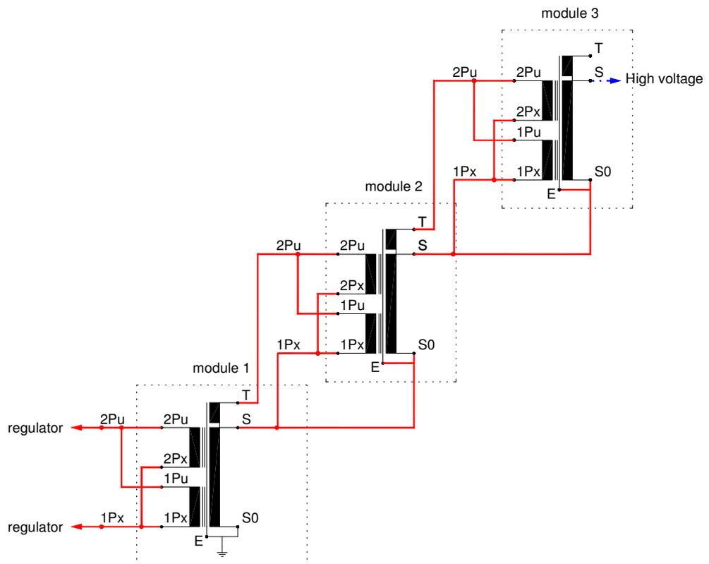
Fig. 62a: Schematic diagram for cascade connection of three test transformers
