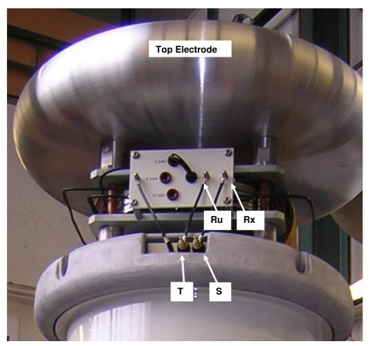
Fig. 61c: Connections between the last module and compensating reactor
