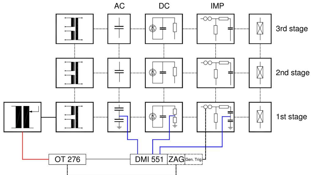
Fig. 1: Block diagram of high voltage construction KIT
