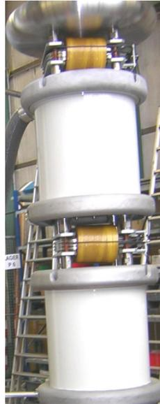
Fig. 7: Compensating reactor
