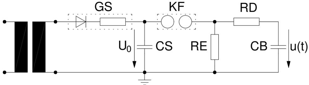
Fig. 51: Circuit for generating impulse voltages
