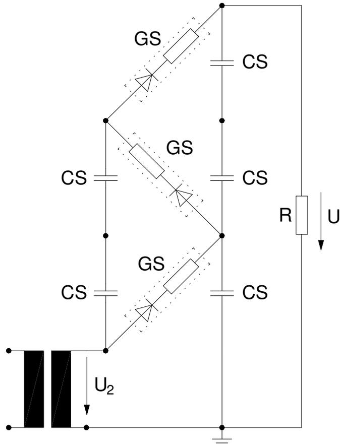
Fig. 48: Greinacher Cascade Circuit with three stages
