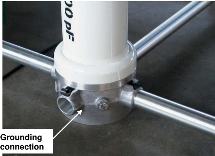
Fig. 3: Floor pedestal with one KIT component and spacer bars
