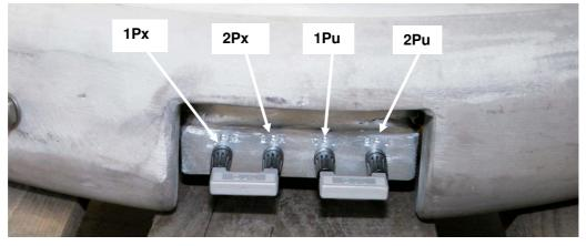
Fig. 59: Parallel connection of primary windings
