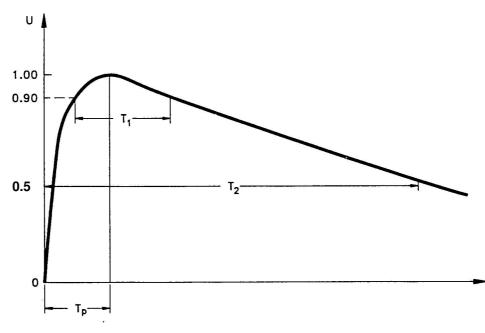
Fig. 50. Switching impulse curve
