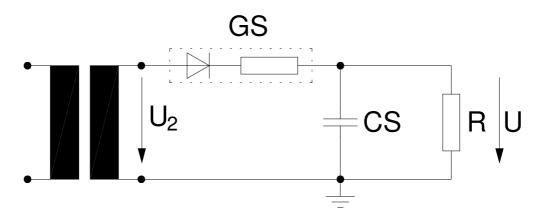
Fig. 44: Half-wave rectifier
