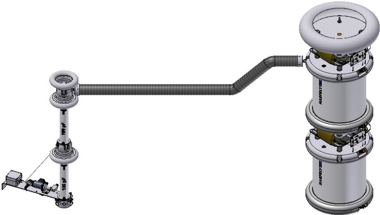
Fig. 64: Build-up AC configuration 2 stages
