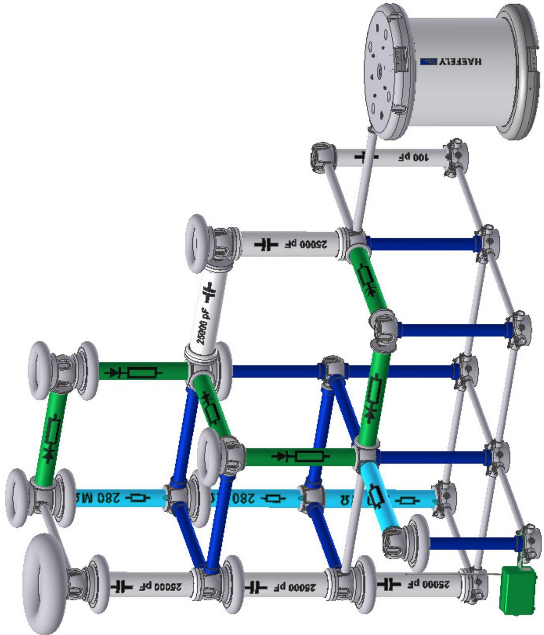
Fig. 68: Build-up DC configuration 3 stages
