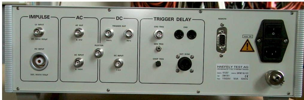
Fig. 43a: Rear side of DMI551 with measuring channels
