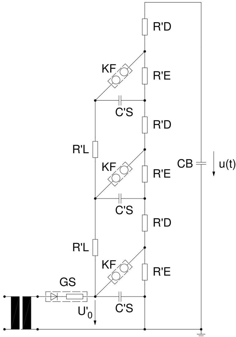
Fig. 53: Multiplier circuit for Impulse 3 stages
