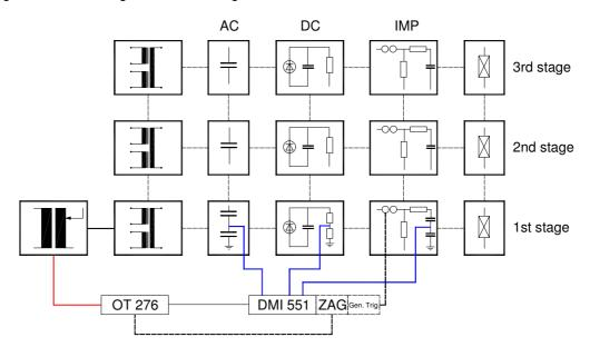
Fig. 1: Block diagram of high voltage construction KIT
