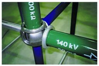
Fig. 2: Connection cup for connecting the KIT components
