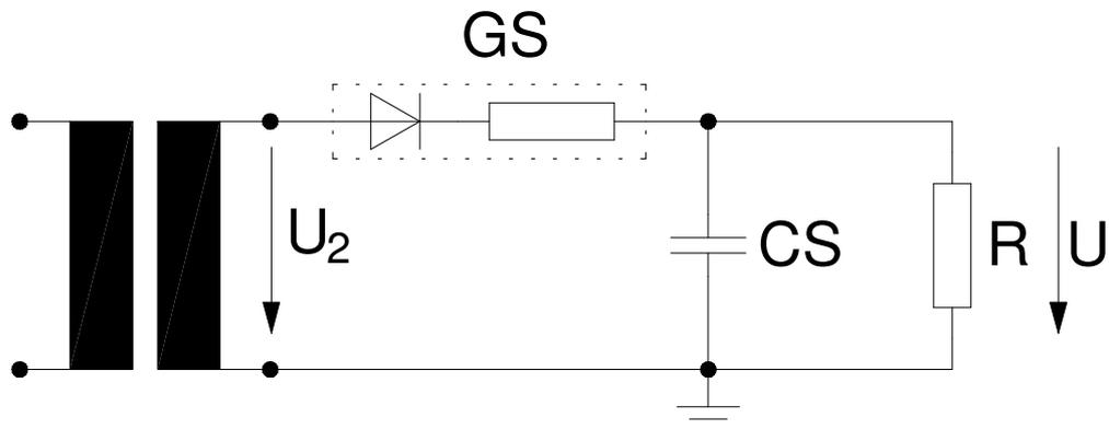
Fig. 44: Half-wave rectifier
