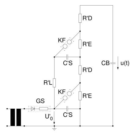
Fig. 52: Multiplier circuit for Impulse 2 stages
