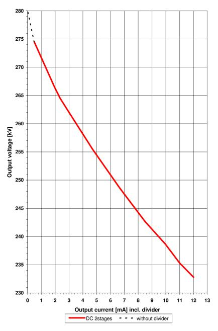
Diagram 3: Load range DC 2 stages With divider an output voltage of approx. 274kV is possible.
