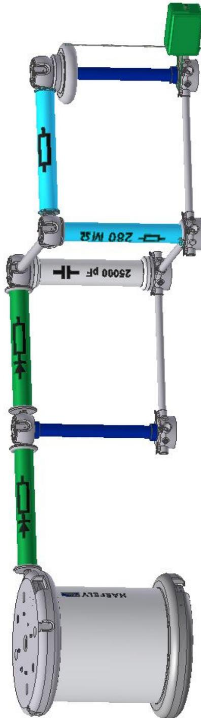
Fig 66: Build-up DC configuration 1 stage
