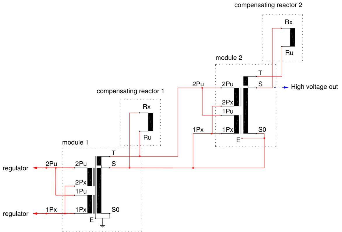
Fig. 58b: Schematic 2 stages with compensating reactors
