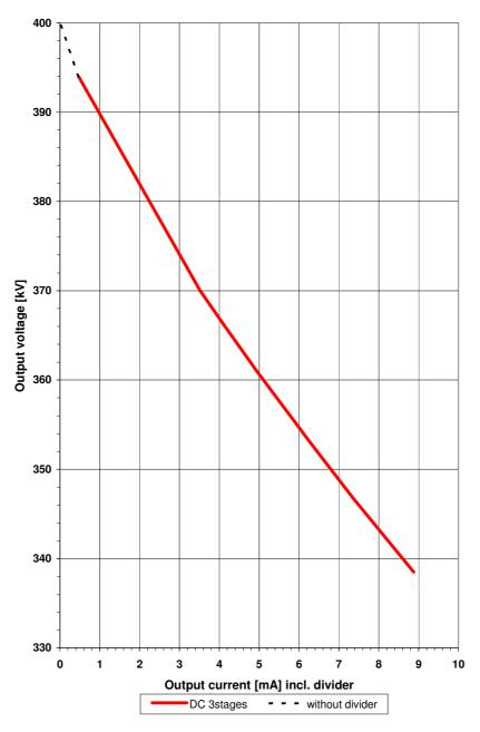
Diagram 5: Load range DC 3 stages With divider an output voltage of approx. 394kV is possible.
