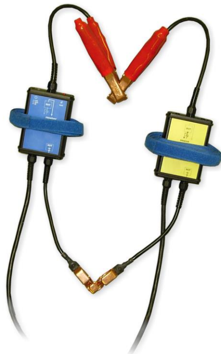
Figure 9 : Shorted Probes for check
