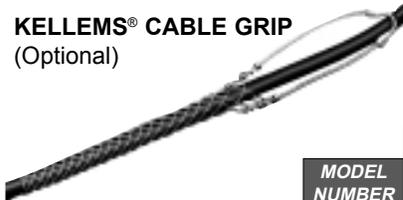
Stocking-type support prevents excessive strain on cable or pullout at connection point. Also absorb additional strain caused by flexure, vibration, expansion and contraction.
