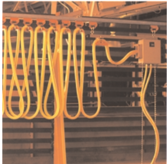
ON THE COVER: Typical Gleason C-Rail festoon system providing traveling pendant control to an overhead crane.
