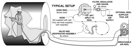
FIGURE CLEAN AIR REELS include stainless steel air path. Also includes ball stop and ratchet lock. Finish is OSHA safety blue baked-on polyester. 3/4"-16 UNF fitting to fit MSA #455022 hose or equivalent. Does not include hose.
