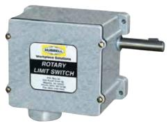
Series 54 switches are designed to serve as pilot controls for magnetic reversing starters and contactors which in turn make and break full voltage between line and load. Contacts in the switch are operated when the external shaft is rotated. For the switch to perform a pilot control function, the contact must be wired in series with the coil circuit of a magnetic reversing starter or contactor.
