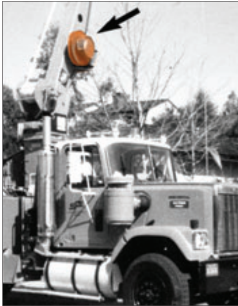
GLEASON K-REEL installed on a hoist.
