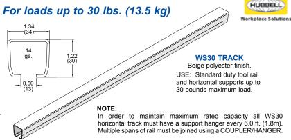
Separate **TOOL RAIL COMPONENTS** allow you to quickly and inexpensively build your own work stations, retrofit existing stations or customize a kit. Finished as shown, all parts are the same high quality included with kits and guaranteed to be interchangeable. Components shown are designed for use with **WS30** rail. Starred (\*) items may also be used with WS50 or extruded aluminum rails. **Mounting hardware, where required, is included.**
