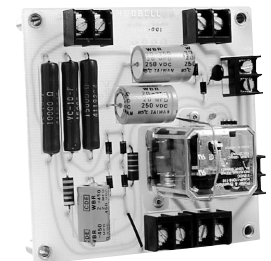
TCA Terminals and Relay Location. (Outline above, photograph below)
