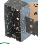
Face mounts on front edge of wood stud. Use when space between studs is limited. (1-3/8" offset)
