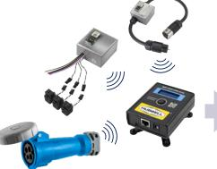
The ethernet gateway gathers data from all connected devices through a wireless mesh network and sends it to the user's front end dashboard for analysis.
