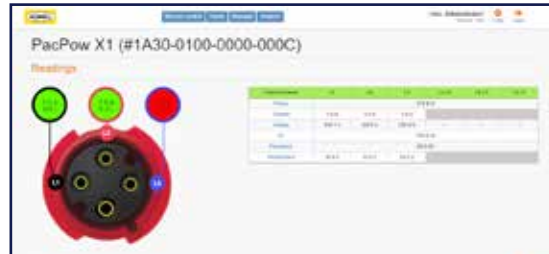
Dashboard displays data sent by the device through the gateway. This example shows one phase of the connector heating up.
