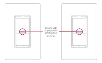
Locate the Primary Switch. Hold "6" until the LED rapidly flashes blue (3 seconds) then release. Next tap "1" to enter pairing mode. The LED will slowly flash blue.
