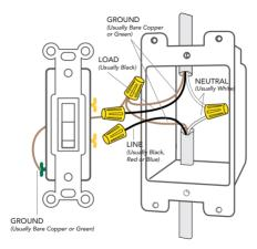
Turn the power back ON at the breaker. Using your voltage detector, identify which of the two wires you removed is energized. This is the "line" wire. The wire that is not energized is the "load" wire. Note these two wires for future reference.
