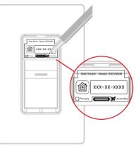
Extend the pull out tab on the front of the Wall Switch connected to the load wire (identified in step 5). Using a ballpoint pen, put an "X" in the box to indicate that this is the Primary Switch.
