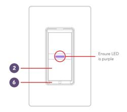
Launch the iDevices<sup>®</sup> Connected app and you will be guided through the process of connecting your Wall Switch. For iOS devices, you will need the HomeKit<sup>™</sup> setup code on the pull out tab on your Wall Switch.
