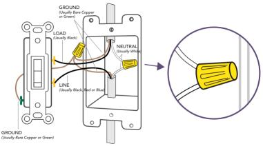
Remove both wires from the terminals of the existing switch and cap with the provided wire nuts. Note: If you have more than two wires connected to your switch (not including the bare copper or green-coated ground wire), please see the 3-way, 4-way installation instructions. It is not necessary to remove the ground wire.
