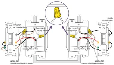
Remove the wires from the common terminal on both of the existing switches and cap with the provided wire nuts. Note: The common terminals usually have a screw that is either black or copper in color.
