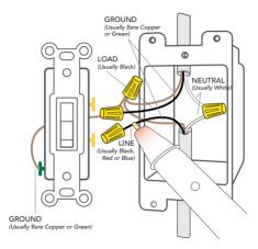
Turn the power back OFF at the breaker and install the iDevices<sup>®</sup> Wall Switch according to the diagram. Ensure all wire nuts are securely fastened.
