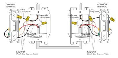
Turn the power back ON at the breaker. Using your voltage detector, identify which of the two wires you removed from the common terminal is energized. This is the "line" wire. Mark this wire as the Secondary (S) Switch Position. You will need to refer to this during the **Wireless Communication Setup**.
