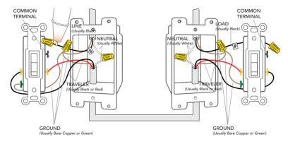
Install the iDevices<sup>®</sup> Wall Switches according to the diagram. Ensure the wire nuts are securely fastened.
