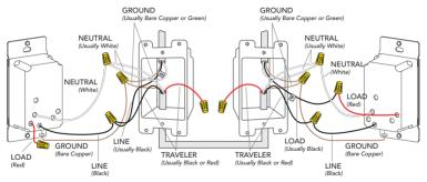
Ensure you install a wire nut on the red wire on the Secondary Switch as well as on both ends of the unused traveler wire (typically red wire)
