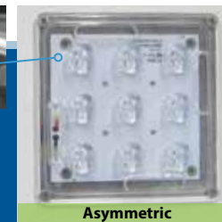
Symmetric lens installed as standard. Rotatable asymmetric lens included with DDL-9L – easily exchangeable by removing four phillips head screws. Lenses are field rotatable in 90° increments.
