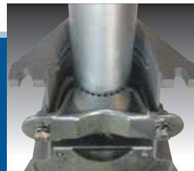
Mast arm clamp easily adjusts to 1-5/8" OD arms with two 3/8" bolts
