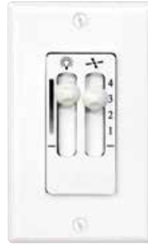
P2630-30 White Four-speed fan wall control with full-range light dimmer. Fits single-gang wall box; requires two circuits. Includes switch plate cover. Not for use with multiple fans.
