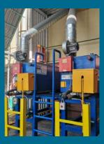
In 2022, our facility in Juarez, Mexico deployed new machinery that reduces hazardous waste by evaporating water content within the waste stream. The new equipment has reduced hazardous waste by approximately 60 tons per month, which in
