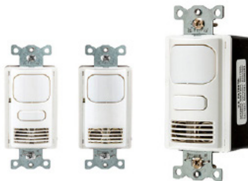
Adaptive Technology Wall Switch Sensors Dual (Ultrasonic and Passive Infrared) 800W Incandescent/Electronic Ballast, 5A LED, 1/6 HP at 120V AC, 1800W Electronic Ballast, 5A LED, 1/6 HP at 277V AC.
