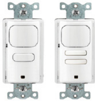
Adaptive Technology Wall Switch Sensors Passive Infrared 800W Incandescent/Electronic Ballast, 5A LED, 1/6 HP at 120V AC, 1800W Electronic Ballast, 5A LED, 1/6 HP at 277V AC.
