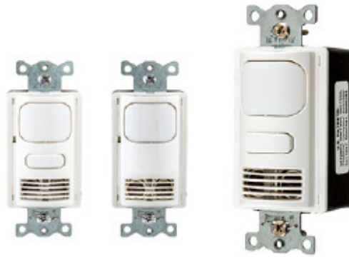
Adaptive Technology Wall Switch Sensors Dual (Ultrasonic and Passive Infrared) 800W Incandescent/Electronic Ballast, 8A LED, 1/6 HP at 120V AC, 1800W Electronic Ballast, 5A LED, 1/6 HP at 277V AC.
