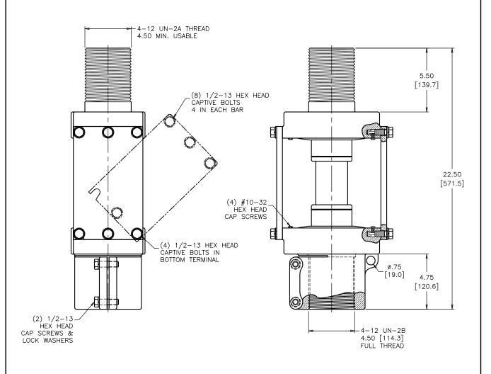
BOLTS ARE EVERDUR AND STAINLESS STEEL HARDWARE IS HIGH CONDUCTIVITY COPPER — SILVER PLATED
