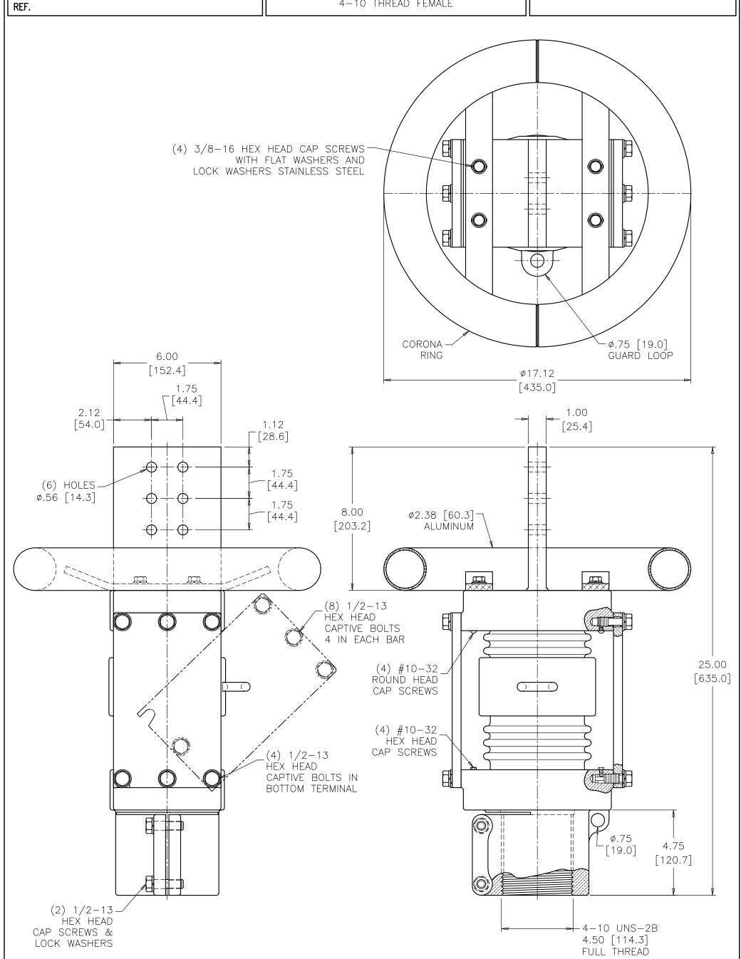
BOLTS ARE EVERDUR AND STAINLESS STEEL HARDWARE IS HIGH CONDUCTIVITY COPPER - SILVER PLATED
