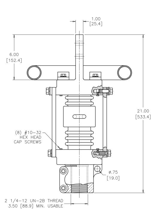
BOLTS ARE EVERDUR AND STAINLESS STEEL HARDWARE IS HIGH CONDUCTIVITY COPPER - SILVER PLATED
