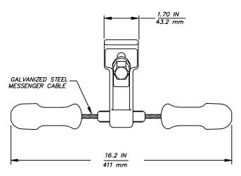
CONDUCTOR RANGE: .385 IN TO .865 IN (6.8 mm TO 22.0 mm)
