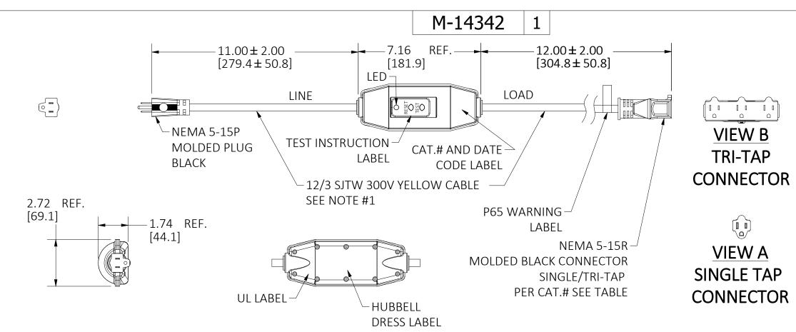
LIST OF PARTS DESCRIPTION **MATERIAL FINISH** HOUSING THERMOPLASTIC BLACK BLADES BRASS GROMMFT ELASTOMER **BLACK** STRAIN RELIEF STEEL ZINC PLATED **SCREWS** STEEL ZINC PLATED **CORD** PVC **YELLOW** RECEPTACLE THERMOPLASTIC BLACK
