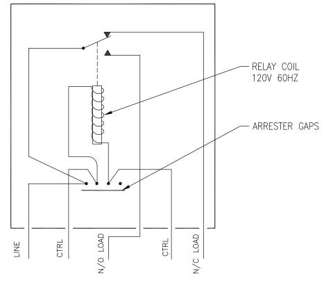
SPDT 30 AMP LOAD 120 VOLT AC W/ 120 VOLT 60HZ COIL
