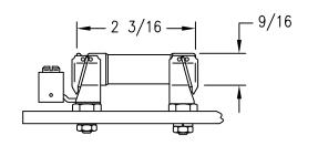
FUSE - DUAL ELEMENT, TIME DELAY, CLASS RK5 - 250V/60A
