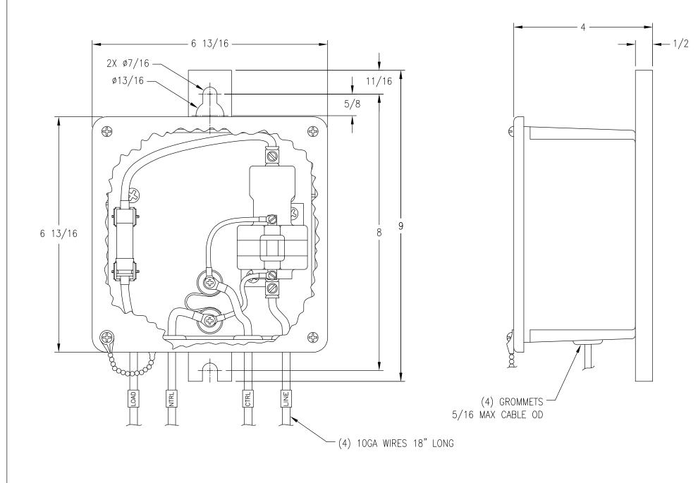
RELAY COIL -120V WEATHERPROOF CASE LOAD CONTACTS NORMALLY OPEN WHEN COIL IS DE-ENERGIZED 30 AMP 250V FUSE -DUAL EXPULSION GAP CONTROL CIRCUIT LIGHTNING ARRESTERS W/ SPRING CLIP MOUNT BROKEN LINES IDENTIFY -CONNECTIONS TO FOUR LEADS EXTENDED FROM LOWER CASE WALL 120V LOAD LEAD 120V LINE LEAD
