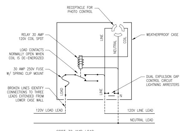
SPDT 30 AMP LOAD 120 VOLT AC W/ 120 VOLT 60HZ COIL
