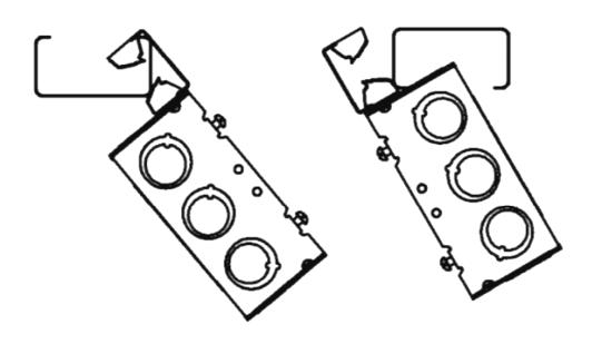
Engage bracket to open side of stud and hinge box into position.
