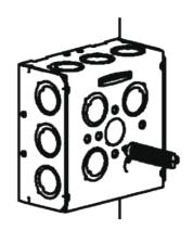
Snap Far Side Box Support into hole in back of box. Support suited for 1-1/2" deep box in 3-1/2" wall.
