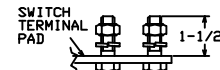
OPTION "C" CAPTIVE HARDWARE CONSIST OF 4 EACH: 1/2" STAINLESS STEEL BOLTS, LOCKWASHERS, & NUTS
