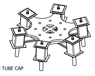
SQUARE TUBE FILLED WITH NONSHRINK GROUT MINIMUM 4000 PSI COMPRESSIVE STRENGTH \*PROVIDED BY OTHERS\*
