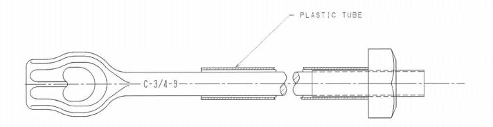
CONFIDENTIAL: THIS DRAWING AND 115 CONTENTS ARE CONFIDENTIAL AND THE EXCLUSIVE COMPIES MAY BE MADE WITHOUT WRITTEN CONSERVED UNDER THE COMPUNIT ON OPERATOR OF HUBBELL / A. B. CHANCE COMPANY. REV. DATE CHANGED BY LATEST EC NO: 91082804 KOEHLER 00-20-91 THREADED TWINEYE ROD 3/4"
