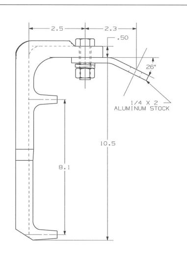
1/2 X 1-1/2 HH. MACHINE BOLT W/ LOCK WASHER AND HEX NUT 9/16 SQUARE -NOTES-1. MATERIAL: ALUMINUM 2. EACH CABLE POSITIONER COMES WITH CABLE WRAP, ADHESIVE PAD, AND WRAP CLAMPS. 3. ACCOMODATES 3/4" TO 3" O.D. CABLE.
