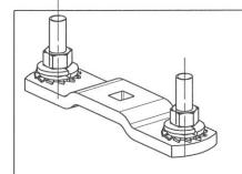
1. MATERIAL: HOT ROLLED STEEL PER ASTM A663.
