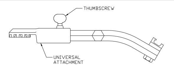
USED TO INSTALL COTTER KEYS INTO SIMI-RECESSED HARDWARE SUCH AS FOUND ON EHV, THIS TOOL WILL HOLD THE KEYS IN POSITION FOR PROPER INSERTION INTO CLEVIS PINS. THE TOOL WILL HOLD THE KEY FIRMLY, YET READILY RELEASE ONCE ENGAGEMENT IS MADE.
