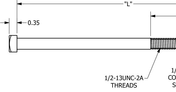
BOLT HEADS WILL HAVE MANUFACTURER'S ID MARK AND A "CW" MARK FOR COLD WEATHER APPROVED BOLTS
