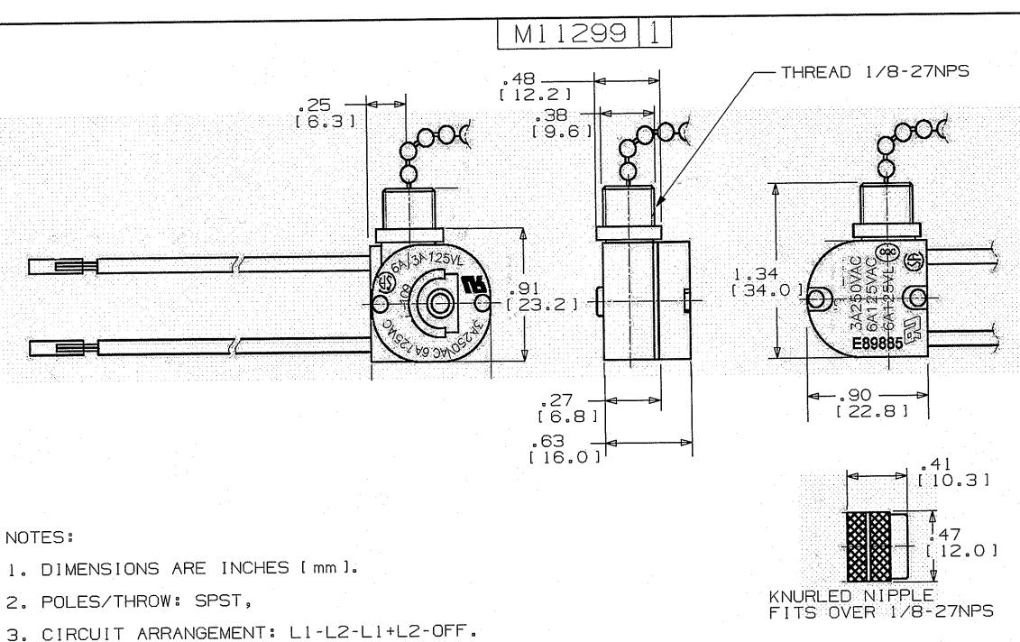
12/01/09 RELEASE TO CAC PRODUCTION PER DCN 16198 REVISIONS THE DESIGN AND DIMENSIONS OF THE PRODUCT SHOWN ON THIS DRAWING ARE SUBJECT TO CHANGE WITHOUT NOTICE TITLE SPECIAL USE SWITCH PULL CHAIN, 2 CIRC, WIRING DEVICE-KELLEMS TOLERANCES UNLESS HUBBELL INCORPORATED OTHERWISE SPECIFIED BRIDGEPORT, CT
