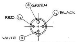
VIEW SHOWING WIRING OF CONNECTOR (COVER NOT SHOWN)
