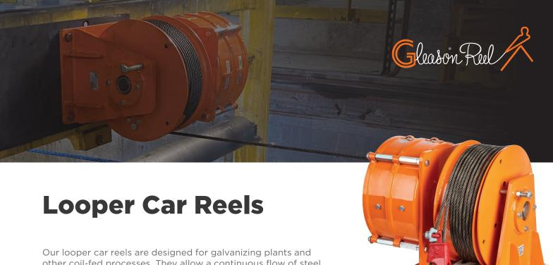
other coil-fed processes. They allow a continuous flow of steel while a full coil is being inserted or removed.
