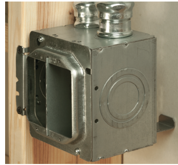
Use standard 4-11/16" sq. covers and 981 partition for power and data in same box
