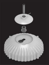
Slide top cover up onto conduit. Screw threaded knob on bottom of conduit.
