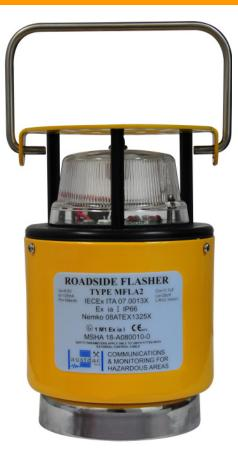
The MFLA2 may also be provided with an attached control lead to allow the flasher to be controlled by a set of voltage free contacts such as those on a pressure or level switch. This external control allows the MFLA2 to be used in 'non-powered' alarm and warning annunciation applications throughout an underground mine.
