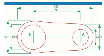
The Anemometer has a bracket with a 25mm (1 inch) diameter mounting hole to secure it (labelled A on the diagram above). It should be mounted upright, with the cable entry at the top of the unit.
