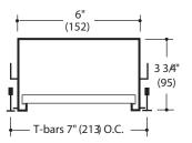
Light opening is framed by wall angles and a main tee spaced 7 1/2" from wall. Horizontal flange of wall angle should be 15/16". Corners are not available for wall-mount systems.
